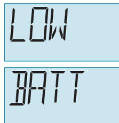
Figure 3-3 Alarme LOW BATT (pile faible)
