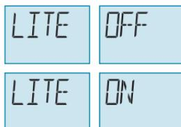
*Figure 2-30 Backlight Settings LITE OFF and LITE ON*
