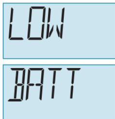
Figure 3-3 LOW BATT Alarm
